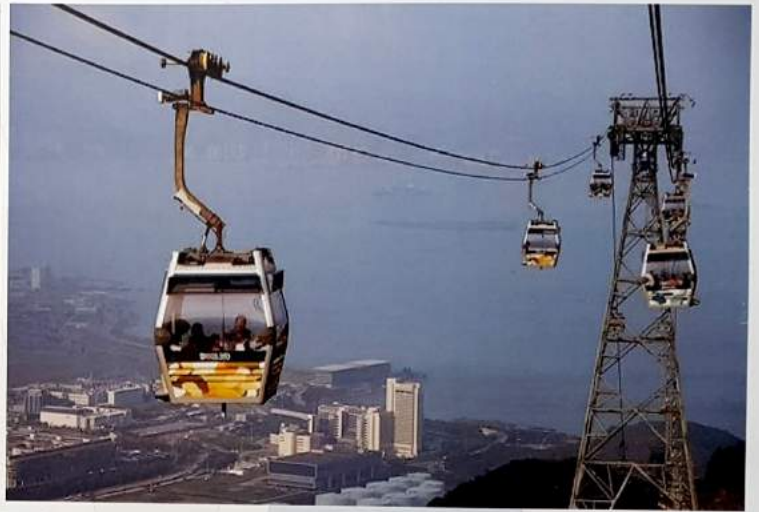
BI CABLE GONDOLA SYSTEM WITH GONDOLA CAPACITY OF 6 PERSONS
